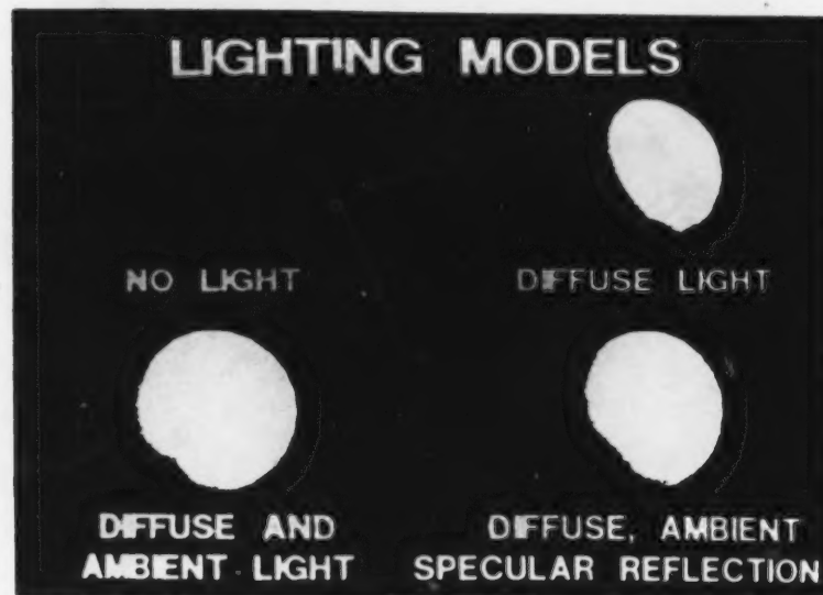
Figure 47. Lighting models; diffuse, ambient, and specular reflection
