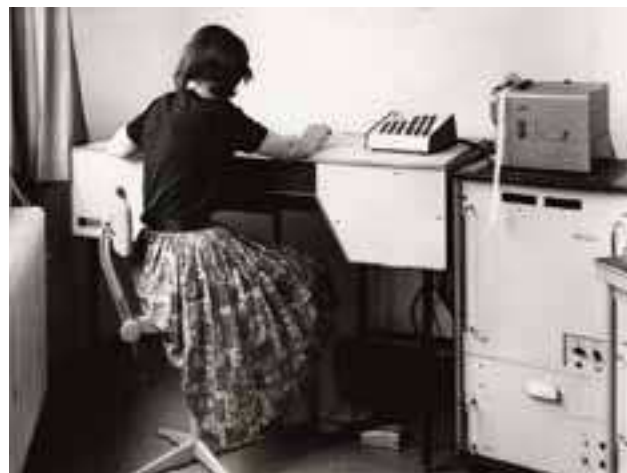
Digitizer or antiplotter, with the foot pedal (the forerunner of the mouse) for the De Telefunken TR4 from 1964 in Groningen.
