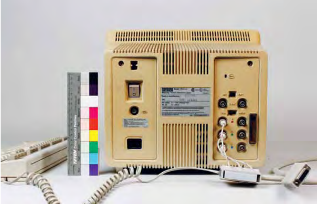
Cable labeled BCC03; it serves probably as monitor cable as well as port for the keyboard. Photograph taken for documentation purposes
