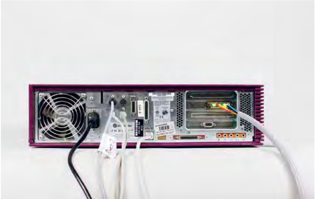
Back of the SGI Indigo2 workstation with the appropriate cable connections Photograph taken for documentation purposes Photo © ZKM | Karlsruhe
