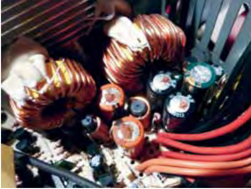
Defective capacitor in the main supply circuit of a computer © PACKED vzw
