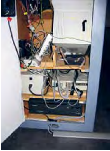
Open console of the installation Karlsruhe Moviemap (version 1991) The components originally used are easily identifiable: the Apple Macintosh Portrait Display (above), the Apple Macintosh IIx and the Pioneer laser disc player LD-V8000 by (below). Photo © ZKM | Karlsruhe
