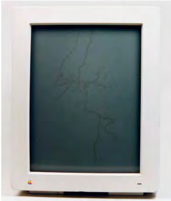
The defective Apple Macintosh Portrait Display (screen burn-in) Photograph taken for documentation purposes Photo © ZKM | Karlsruhe
