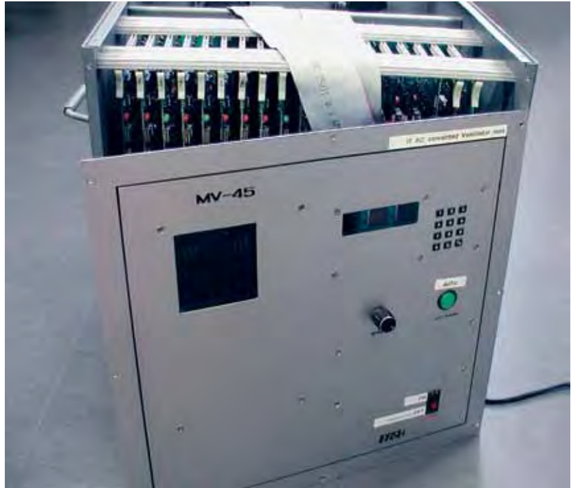
The so-called split screen generator MV-45 is a custom-made system by DASH Systems. Photo © ZKM | Karlsruhe
