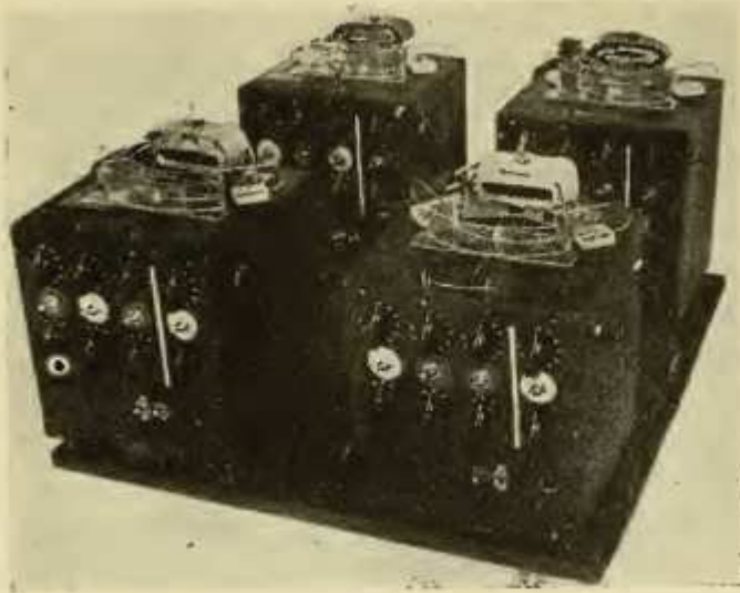
FIGURE 8/2/1 : The Homeostat. Each unit carries on top a magnet and coil such as that shown in Figure 8/2/2. Of the controls on the front panel, those of the upper row control the potentiometers, those of the middle row the commutators, and those of the lower row the switches S of Figure 8/2/3.
