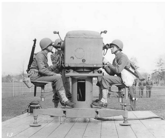
Fig. 9.1. M-9 gun director, tracking head with operators. One follows the target in elevation, the other in azimuth. The unit and the operators rotate while tracking. Courtesy of AT&T Archives.
