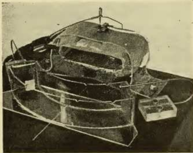
FIGURE 8/2/2 : Typical magnet (just visible), coil, pivot, vane, and water potentiometer with electrodes at each end. The coil is quadruple, consisting of A , B , C and D of Figure 8/2/3.
