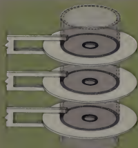
Figure 2. A cylinder is made up of corresponding tracks on the top and bottom surface of each disk in the drive.
