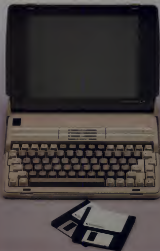
The LCD screen of the DG/One displays 25 lines of 80 characters in the same proportions as a CRT screen.
