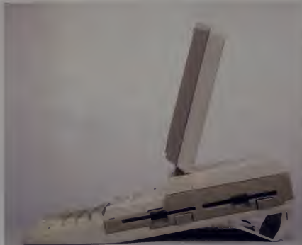
The Data General/One comes with one 3.5" disk drive built in. A second drive is optional.
