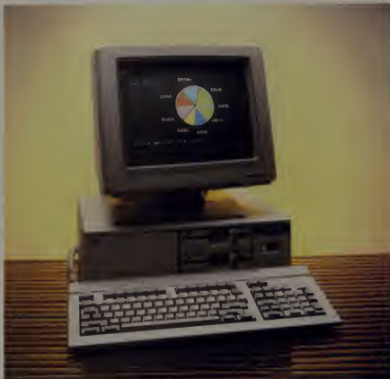
NEC's Advanced Personal Computer offers a 640 x 400 high-resolution display with up to eight colors.
