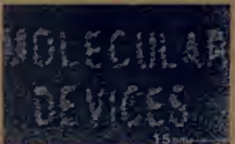
The lettering above was etched in NaCl (table salt) by the electron beam of the STEM. The 15 nanometer scale equals 0.015 microns. At this size, the entire Encyclopedia Britannica could fit on a postage stamp.
