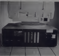
The rear panel of the PC/I. Note the five expansion slots and serial and parallel ports.
