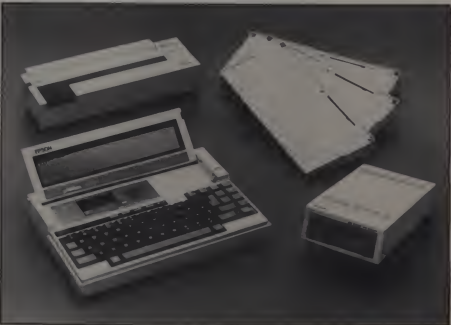
Clip-on thermal printer, RAM packs, the PX-8, and floppy drive.
