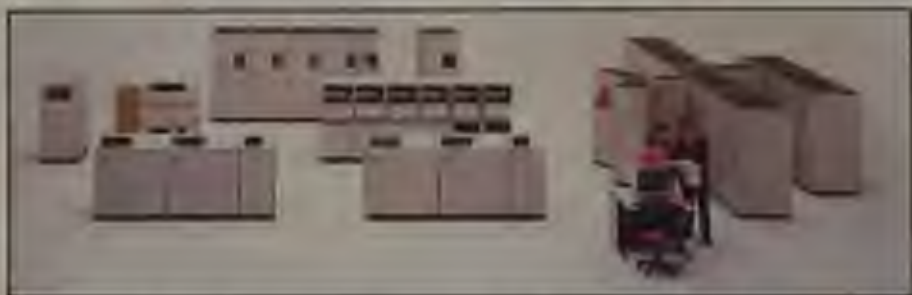
Hitachi S-810 Array Processor supercomputer has a processing speed of 630 floating point operations per second.
