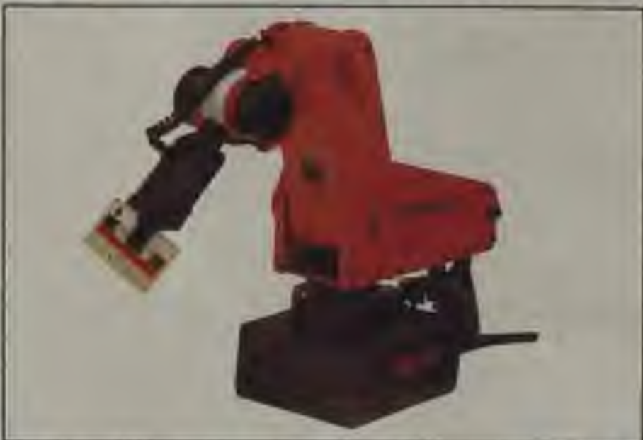
Move Master RM-501 robot comes with an interface box to connect to the RS-232 serial or Centronics parallel port of any personal computer.
