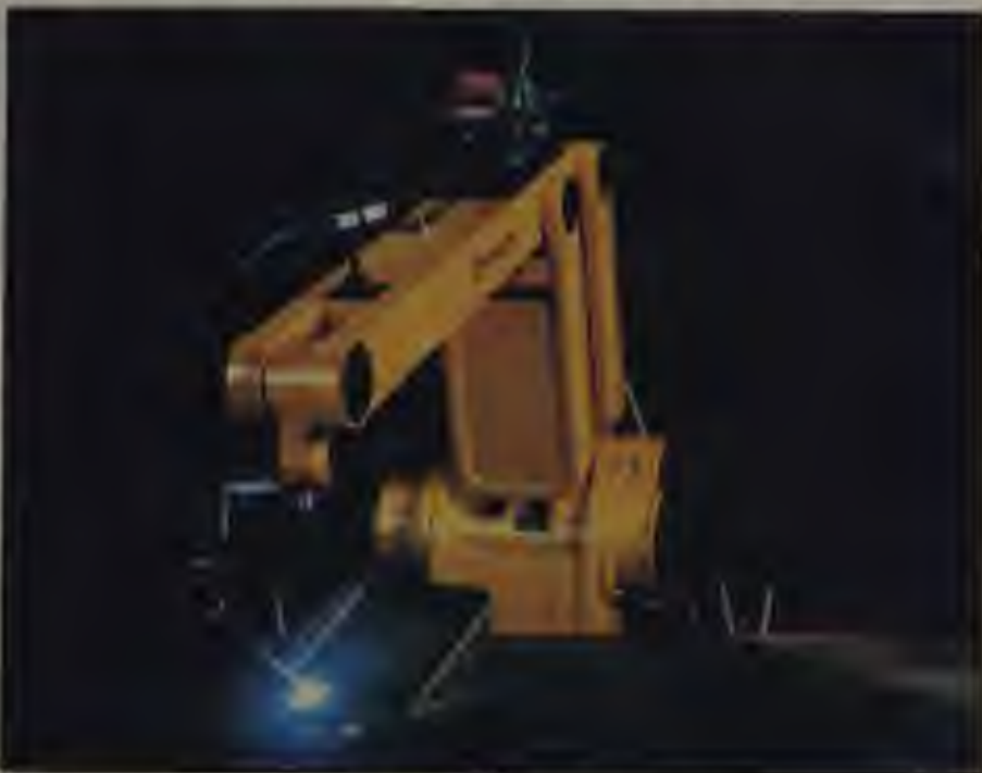
FANUC multi-purpose robot will do arc welding, material handling, assembling, etc.
