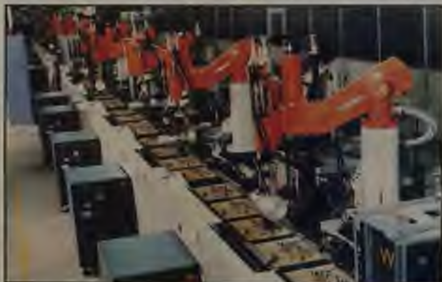
Assembly robots on the color TV production line in Toshiba's Fukaya plant pick up parts and insert them into PC boards.
