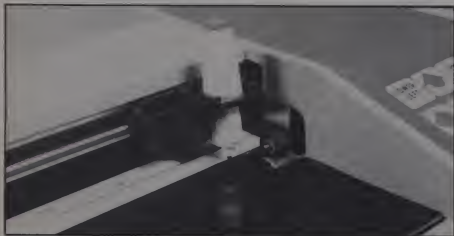
Rollers move the paper back and forth and the pen moves from side to side.
