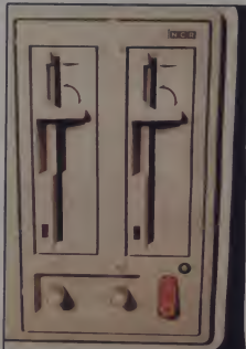
Disks are held in with reliable, quarter-rotation handles. Controls include screen brightness, sound level, and power off/on switch.
