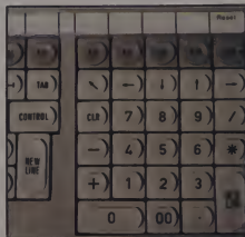
Right side of keyboard has an "extra" CONTROL key above the NEW LINE key. The numeric keypad has double zero for fast entry of financial data. Unfortunately, cursor control keys are arranged in a horizontal line.
