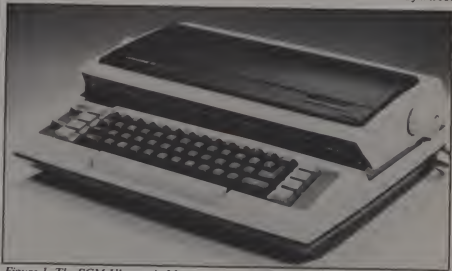
Figure 1. The SCM Ultrasonic Messenger III portable typewriter can also be used as a computer printer: ten printwheels are available in three pitches.
