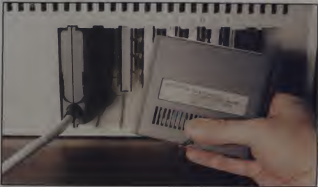
Optional add-ons plug into the back of the unit; no disassembly is required.
