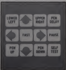
Touch panel on right has 12 plotter controls.
