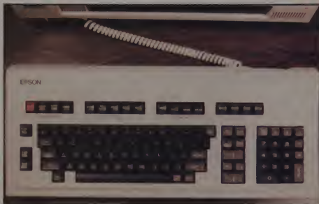
Epson QX-10 keyboard is divided into logical clusters of keys.
