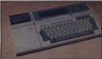
Optional 40-column thermal graphics printer attaches to left side of computer.
