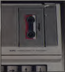
Microcassette recorder operates at 2000 baud; a C-30 cassette can store 128K of data.
