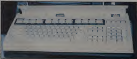
EPS keyboard has PROM modules for use with various software packages.
