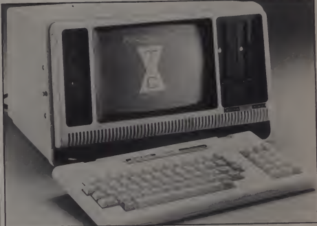
Figure 1. The TRS-80 Model 4P is a transportable version of the Model 4, with thin-line disk drives and a detachable keyboard.
