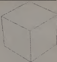
Figure 7. Perspective view of the cube defined by the data in Listing 2. The viewing position was (5,5,5), the focus point was (0,0,0), horizon rotation was 0^\circ , and scaling factor was 6.
