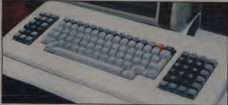
Zicor keyboard has microprocessor and 8K of memory.
