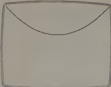
Output from projectile plotter before correcting for vertical distances being measured from the top of the screen downward.
