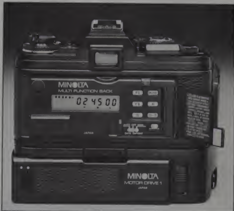
Figure 1. The rear of this Minolta X-700 camera shows two accessories attached: a motor drive and the Multi-Function Back. The control panel cover is open to show the operating keys.
