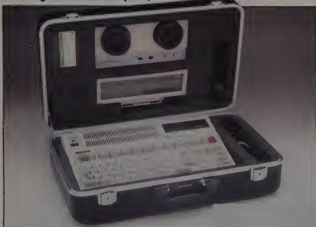
All of the notebook computers fit in an attache case. Here is one of the largest, the Toshiba T100, in a case with LCD display, acoustic modem, memory cartridge, and cables.
