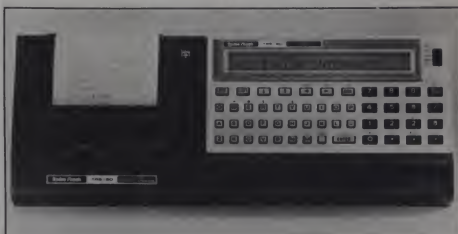
Figure 1. The Pocket PC-3, which fits into a shirt pocket, is shown here plugged into the matching PC-3 printer/cassette interface.
