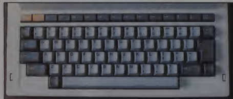
Keyboard has 57 full-stroke keys arranged in a standard pattern, and 15 special keys in a line above.
