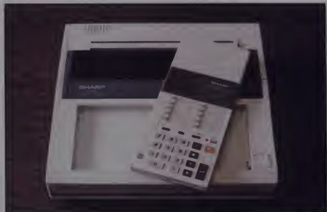
Optional modem fits into the lid of the case. It doubles as a portable conference telephone.
