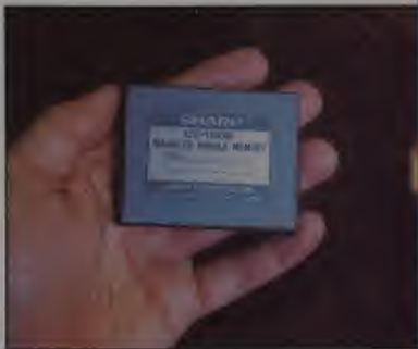
Bubble memory cartridge is just over 2" square.
