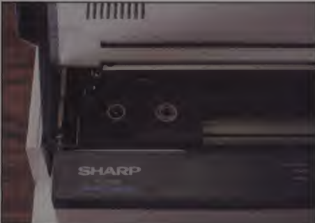
With optional thermal ribbon, the printer can use plain bond paper as well as thermal paper.
