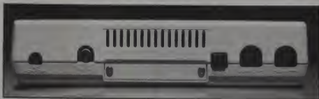
Rear of MC-10 showing (l-r) AC adapter, video out, reset button, serial I/O, and cassette port.
