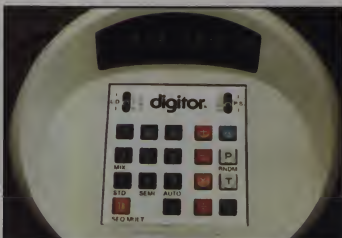
Digitor has green LED characters, ten number keys, nine "programming" keys, and two switches.
