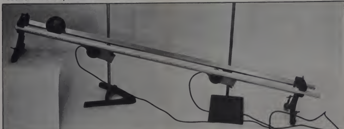
Photo 2. Side view of the velocity/acceleration timer.
