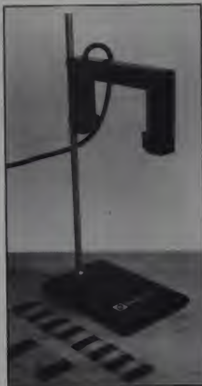
Figure 1. Photogate (infrared light source and detector) and rules used in acceleration experiments.
