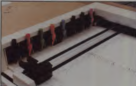
Eight colored pens are held in pen holders at the left of the plotting bed.
