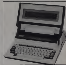
Sharp PC-5000 is a 16-bit portable with 128K, folding display, and optional printer.
