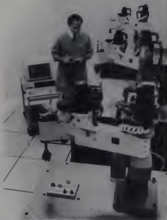
Photo 2. An IBM Personal Computer is used to develop programs for the IBM 7535 Manufacturing System.
