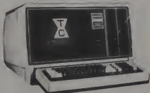
Figure 1. Radio Shack's new TRS-80 Model 16 uses a Motorola 16-bit microprocessor and is compatible with the Model II.
