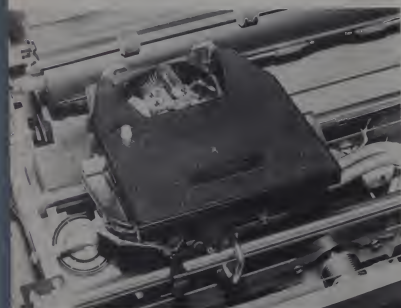
To change the print wheel, ribbon cartridge or character space setting, the entire front cover must be lifted off. A quick glance inside the machine shows it is well constructed.
