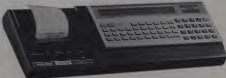
Figure 1. The TRS-80 Pocket Computer easily connects to the printer/cassette interface to provide a compact combination weighing only 1.25 pounds.
