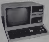
DISK III single drive assembly includes: one 40 track 5 1/4" double density drive, power supply, controller, mounting hardware, and applicable cables.
