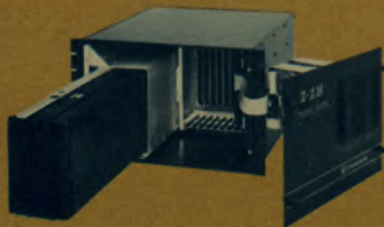
Hard disk drive at lower left can be interchanged just by sliding out and disconnecting plug. Seven free card slots are available. Z-2H includes printer interface card.
