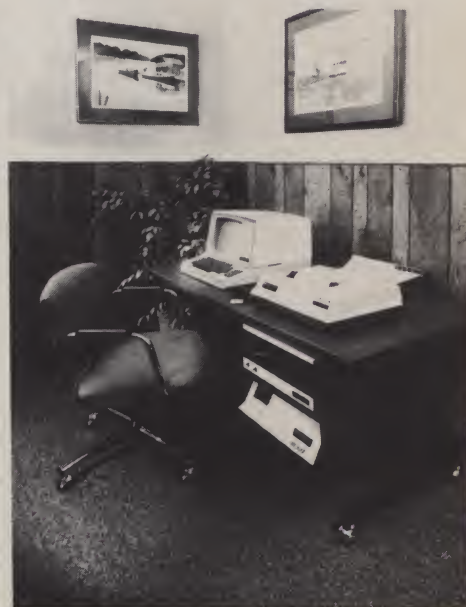
WHS11A minicomputer system consists of the WH11A mainframe (shown in lower right of cabinet); the WH19 microprocessor-based "smart" video terminal (left desktop), and the WH27 dual-drive floppy disk system, (upper cabinet shelf). The system is fully compatible with the DEC PDP 11/03.
