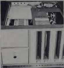
Photo 4. That cardboard over the card cage is completely blocking the air flow to those boards... for 48 hours! Try that with your system ... for 2 hours!
