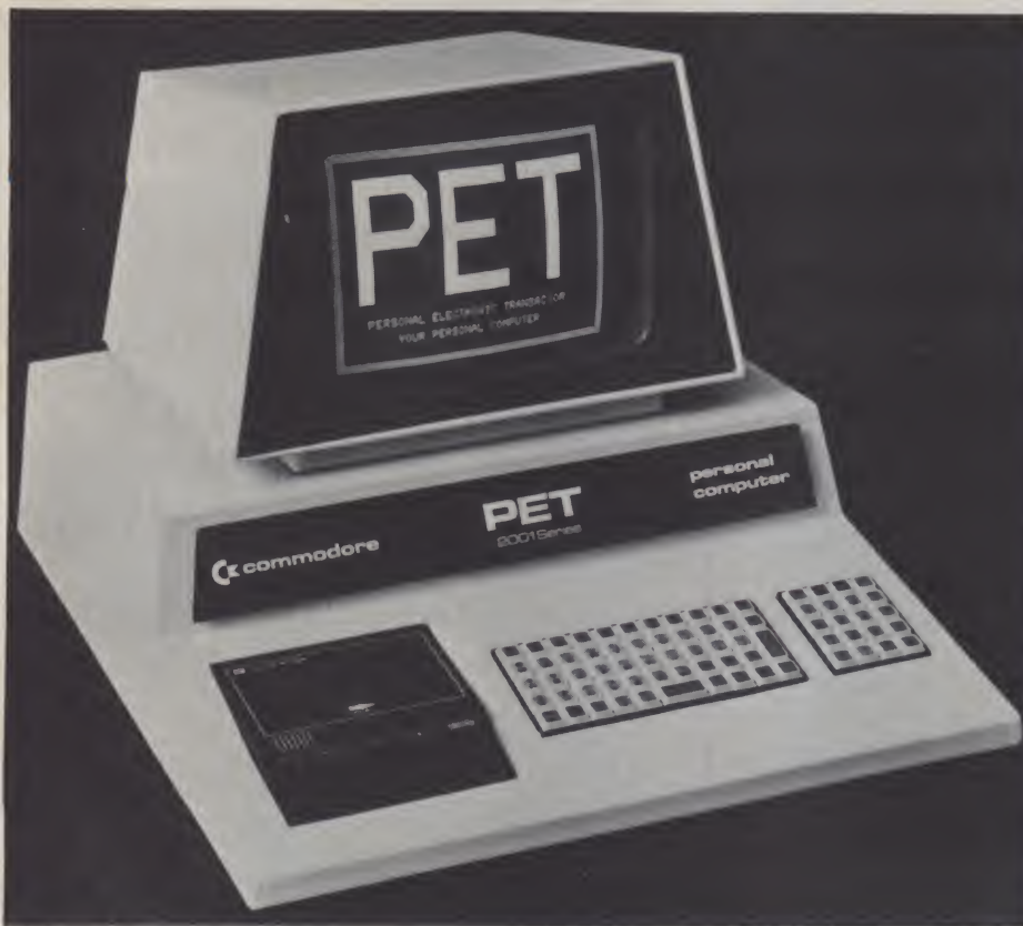
Commodore's PET is one of the very few personal computers that combines all four basic units (keyboard, computer, cassette drive, video output) in a single package.
