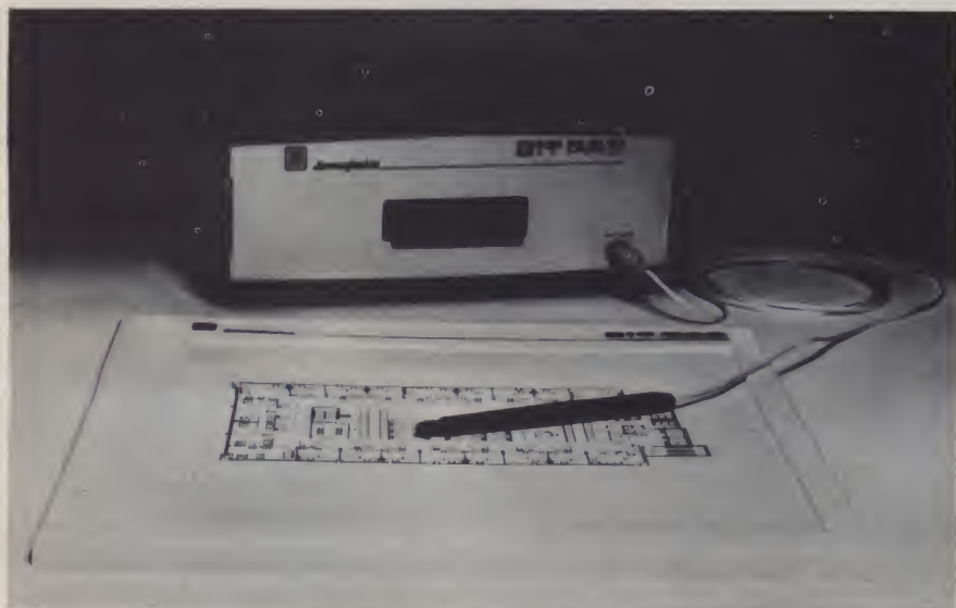
The Bit Pad, with digitizer board, stylus, console cabinet (with controls for selecting the data-collection mode), and RS-232 output, is $555.
