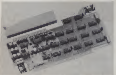
Fig. 4B. Cromemco D+7A analog interface board, used to interface EKG signals with the microcomputer.
