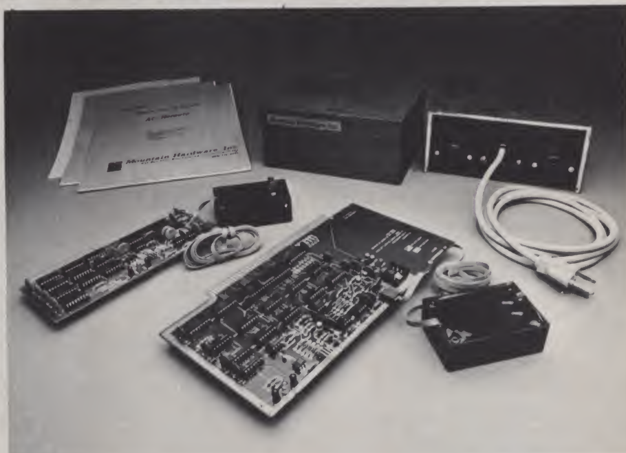
The printed-circuit boards in front are the AC Controllers (Apple II at left, S-100 board at right). Two Dual Channel Remote units are shown in the background.
