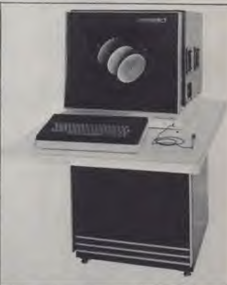
The Vector General Series 3's capabilities range from a simple two-dimensional graphics display to complex 3D transformations including scale, rotation about all three axes and variable intensity for depth cuing.
