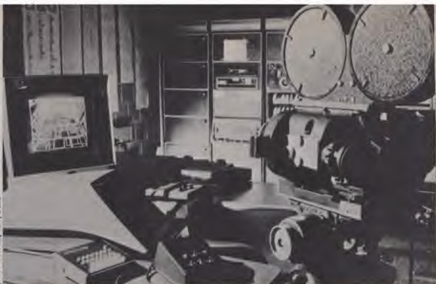
Larry Cuba's setup for the Star Wars computer animation, with the PDP 1145 racked in the rear, the Vector General screen and Mitchell camera.
