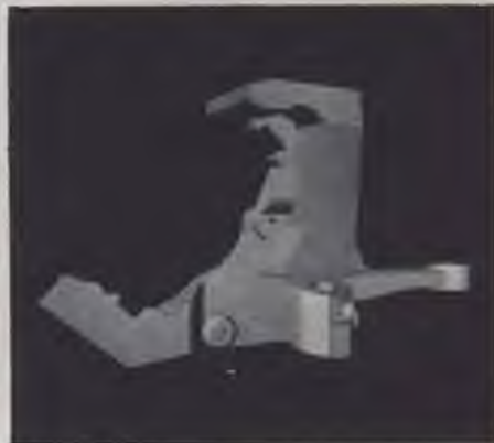
Here you see an 18-mm spindle for the wheel of a car which, once described, can be rotated about a central axis to show other angles. In this case, the spindle was rotated 70 degrees for each picture.
