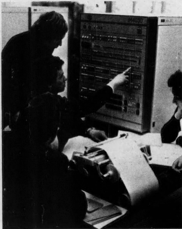
Instructor points to register of Russian M4030 timesharing system.
